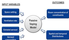
Physics-based models that include fluid flow, mass and heat transfers along with thermodynamic and kinetic interactions
