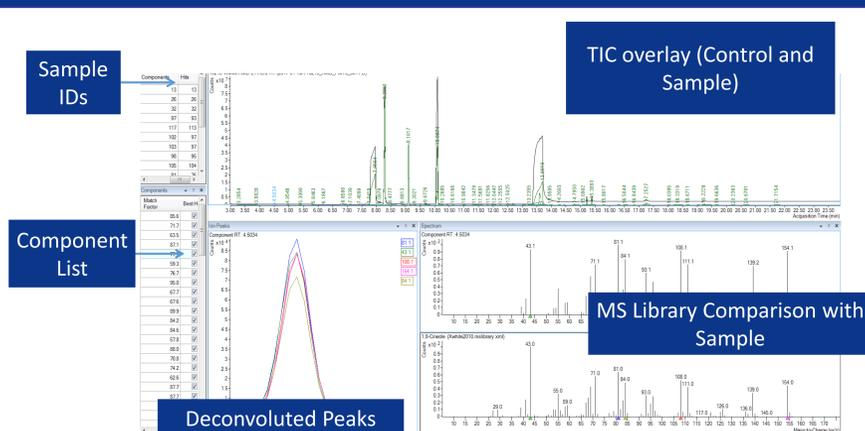
Component table is generated after automatic spectral deconvolution of the peaks and library search. ALCS custom In-house Mass Spectral Library was developed and used for data reprocessing and currently contains > 900 compounds. Identifications are confirmed by mass spectrum match factor, visual inspection of the peak/mass spectrum, and retention time.
