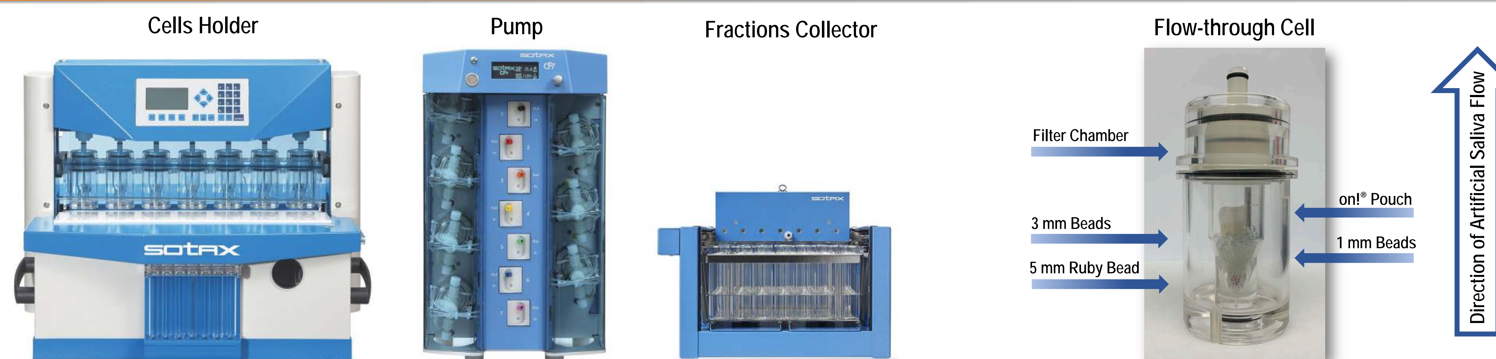
Figure 1. SOTAX CE7 Smart flow-through system (USP-4) including cells holder, pump, fractions collector, and flow-through cell. 5
